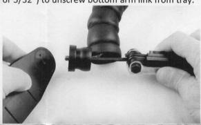
**Step 3:** Using the screw and washers provided, attach the bottom arm link to the Flex-Connect adapter in the order shown below. Use a 3/16" Allen Wrench.
